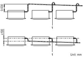
T-joint converging drain pipes
